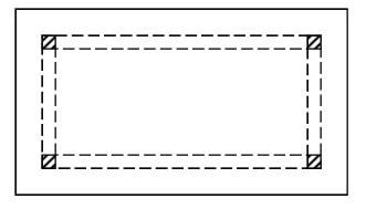
Given that fcu = 35N/mm2, fy = 460N/mm2, cover to main steel is 20mm, estimated diameter of main steel is 8mm and imposed load is 1.5kPa, design and detail the slab.
